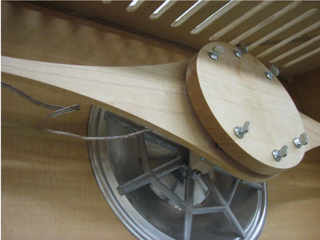
Figure 19: The Resophonic Manta resonator – detail of the aluminum cone
